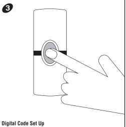
• Press the Push Button once, a new operation code is generated randomly and sent to the Chime unit.
