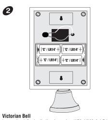
Insert 4 x 1.5volt alkaline batteries ("C", UM2 & LR14 - not included) into the battery compartment at the back of the Bell unit, ensuring the battery polarity matches the internal markings.
